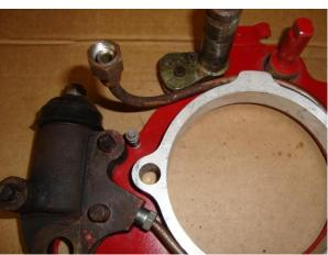
Note the spring retainers snuggling beside the cylinders. They fall out with devilish regularity! Best to have a clean old sheet or something similar to work on to catch the parts that tend to fly off when least expected.
