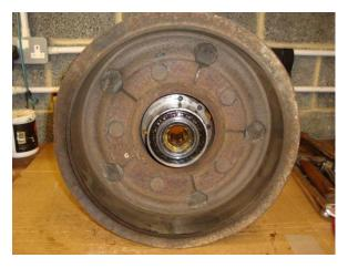
The brake drum from the inside showing the large one piece bearing. This was quite difficult to get back on one the brake assembly had been bolted up. After hammering to no avail with a wooden mallet I bolted up the puller I made and used it in reverse. Make sure the splines from the drive shaft enter the bearing before you try to bang the drum on too far. Once enough of the threaded section of the drive shaft protrudes, use the retaining nut to finish pulling the shaft through and forcing the
