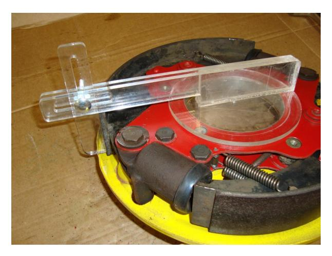
I made this centring tool from Perspex and used it to set the pivot end of the brake shoes to be the same by using the eccentric to adjust movement. The adjusting cams on the back of the assembly are turned so that the shoes are released.
