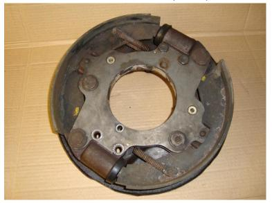
The following two pictures show the shoe side and revers side. On the shoe side the springs can clearly be seen. The circular shapes of the eccentrics are located adjacent to the cylinders on the reverse castellated nuts and split pins that hold them in place. One of the nuts is in a deep recess so the split pin has to be removed by bending and pulling. Undo the nuts and tap out the eccentric retaining bolt but be careful not to damage the
