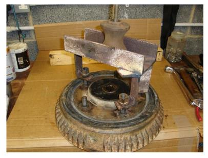
inside. You will need to make a puller. As you can see mine is made of sections of steel channel welded together with a long steel rod threaded and nutted at both ends and a sliding weight. Attach it on three wheel nut locations and bang away until the drum comes free with its bearing. The splined drive shaft will become lose at this point and the universal joint will allow the shaft to be pushed back. This is important in order to remove the pinch bolts that
