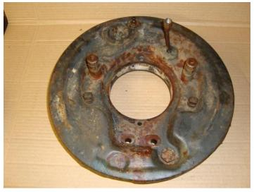
The splined shafts of the hand brake mechanism can be seen on the reverse side as can the brake adjusters. As the assembly is dismantles the splined shafts will come free. The actuating lobes have a wheel held in with a loose pin. Note which was round the lobes are as the mechanism is handed. Take this opportunity to clean everything. Apart from the cylinders and pistons I have used a handful of washing powder dissolved in boiling water and a scrubbing brush to get rid of
