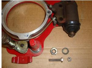
The brake pipe that wraps around the central aluminium spacer does tend to get bent out of shape when you are taking things apart and becomes a real problem when trying to connect up again when the assembly is bolted back to the hub. Be careful not to bend it too much.
