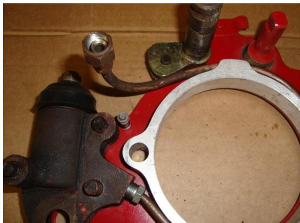
Note the spring retainers snuggling beside the cylinders. They fall out with devilish regularity! Best to have a clean old sheet or something similar to work on to catch the parts that tend to fly off when least expected.
