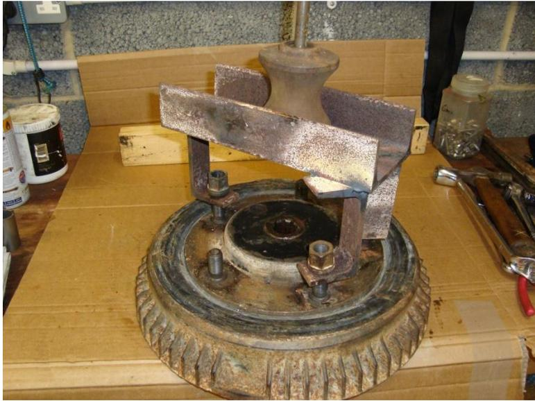
inside. You will need to make a puller. As you can see mine is made of sections of steel channel welded together with a long steel rod threaded and nutted at both ends and a sliding weight. Attach it on three wheel nut locations and bang away until the drum comes free with its bearing. The splined drive shaft will become loose at this point and the universal joint will allow the shaft to be pushed back. This is important in order to remove the pinch bolts that
