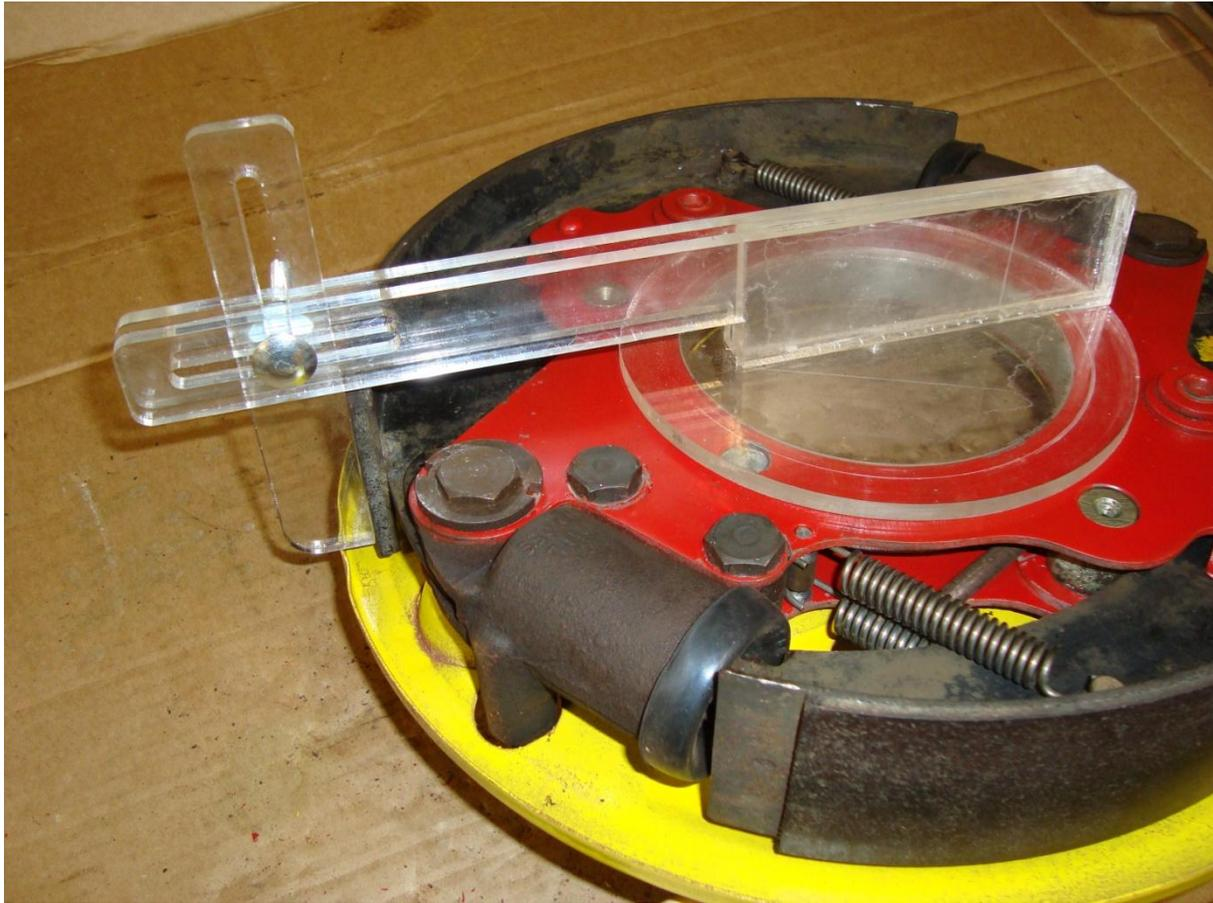
I made this centring tool from Perspex and used it to set the pivot end of the brake shoes to be the same by using the eccentric to adjust movement. The adjusting cams on the back of the assembly are turned so that the shoes are released.
