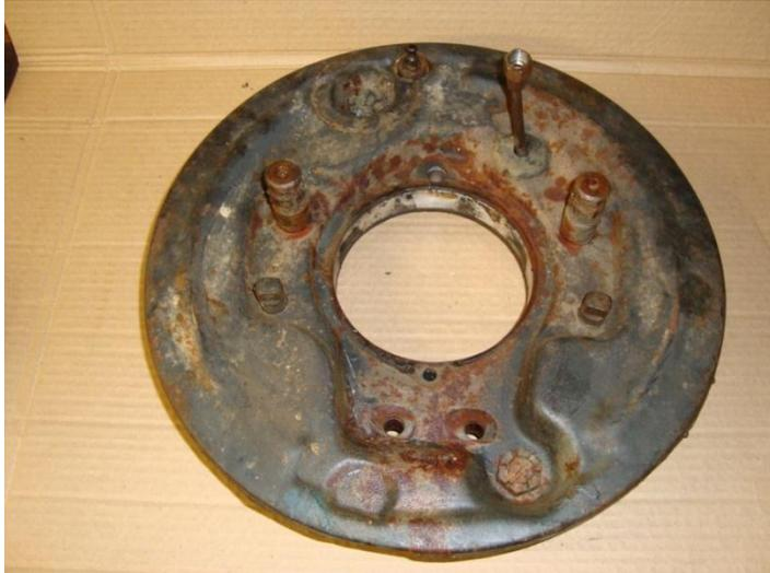
The splined shafts of the hand brake mechanism can be seen on the reverse side as can the brake adjusters. As the assembly is dismantled the splined shafts will come free. The actuating lobes have a wheel held in with a loose pin. Note which way the lobes are as the mechanism is handed. Take this opportunity to clean everything. Apart from the cylinders and pistons I have used a handful of washing powder dissolved in boiling water and a scrubbing brush to get rid of
