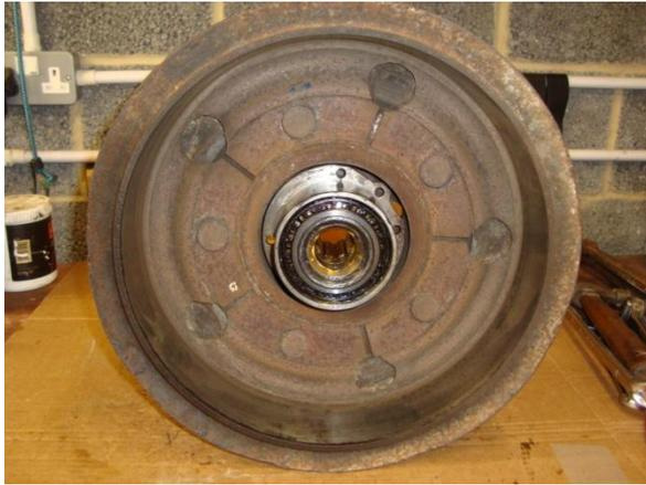
The brake drum from the inside showing the large one piece bearing. This was quite difficult to get back on once the brake assembly had been bolted up. After hammering to no avail with a wooden mallet I bolted up the puller I made and used it in reverse. Make sure the splines from the drive shaft enter the bearing before you try to bang the drum on too far. Once enough of the threaded section of the drive shaft protrudes, use the retaining nut to finish pulling the shaft through and forcing the
