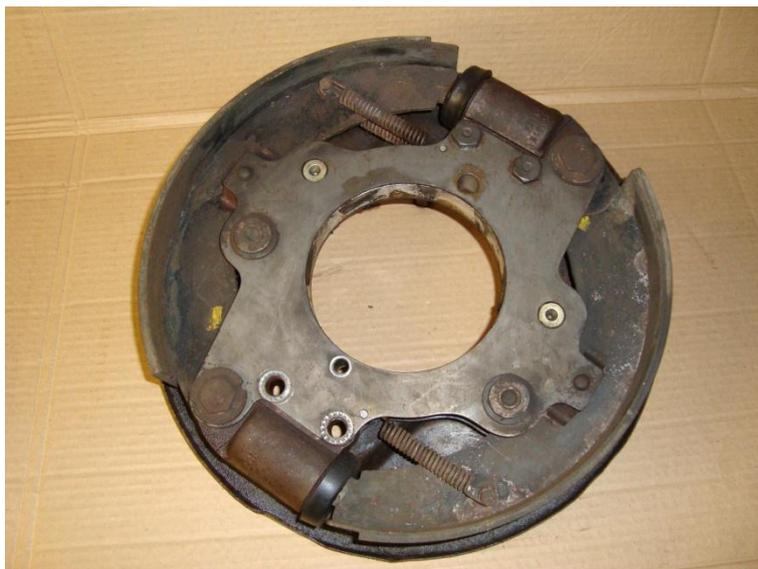
The following two pictures show the shoe side and reverse side. On the shoe side the springs can clearly be seen. The circular shapes of the eccentrics are located adjacent to the cylinders and on the reverse the castellated nuts and split pins that hold them in place. One of the nuts is in a deep recess so the split pin has to be removed by bending and pulling. Undo the nuts and tap out the eccentric retaining bolt but be careful not to damage the threads.
